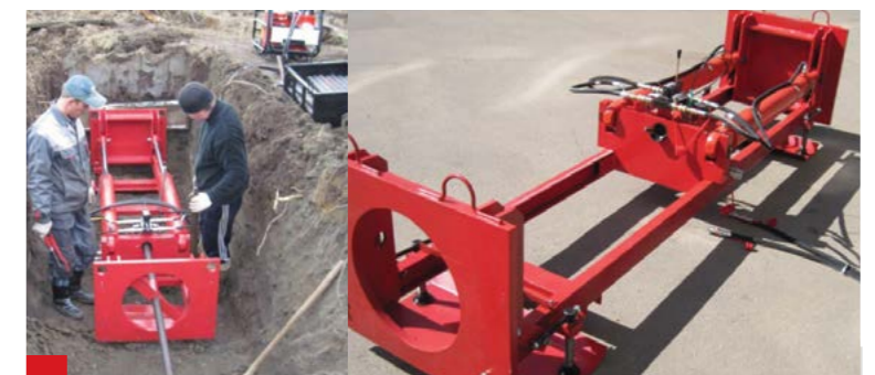
Equipment of a ground puncture – 25U UPG «Arrow» for trenchless installation of underground utilities. Manufacturing and supplying it to companies specializing in the laying of utilities.
