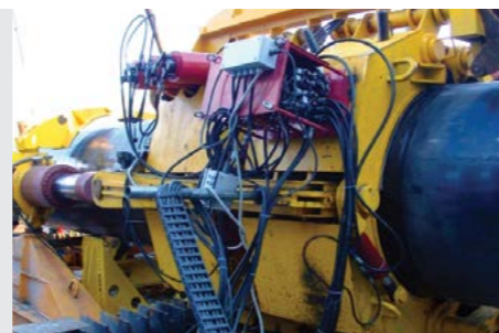
Equipment UPT-700 for pushing pipes in tunnel transition for oil products transportation, Krasnodar region
