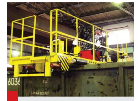
Installation for straightening upper capping frame of gondola wagons UP-2M to «Russian Railways» Inc.
